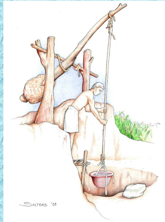
Shaduf ca. 1,700 BC – device for lifting water into canals
